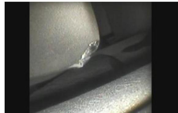
Gambar 1. LP Compressor Stage 1.5 Damage
